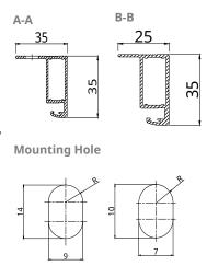
Length: ±2mm Width: ±2mm Height: ±1mm Row Pitch: ±2mm
